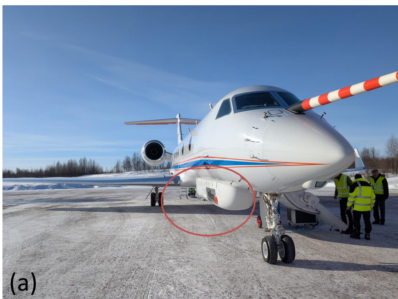
Figure 2. (a) The German HALO research aircraft. The GLORIA instrument (circled) is mounted in the belly pod and observes to the right. (b) HALO in front of the hangar in Kiruna.
